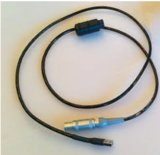
Fig. 17 – Memory readout unit to be connected to the probe and USB outlet of the logging computer.
