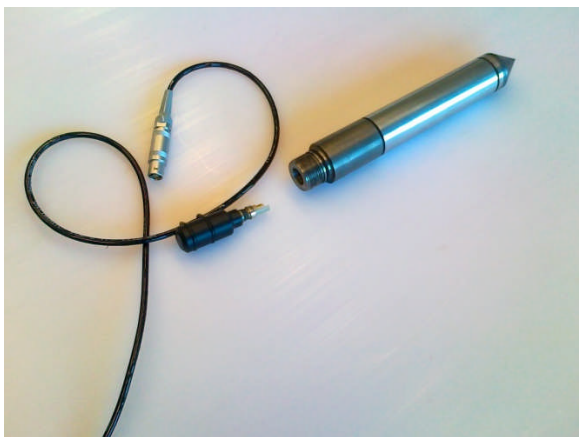
Fig. 33 – Uploading data from memory probe
