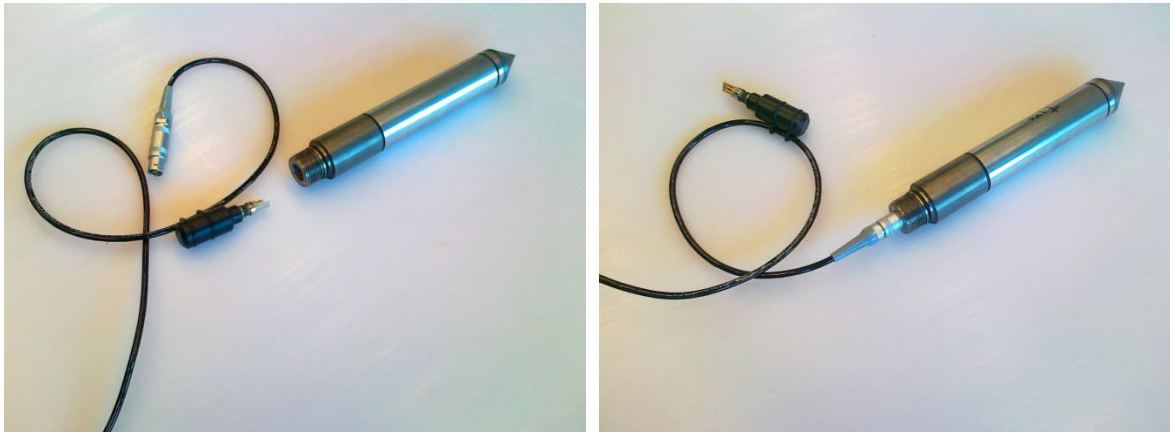
Fig. 22 – Synchronisation of the memory probe before test.
