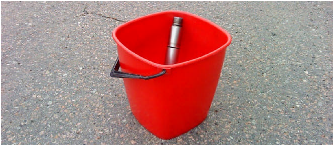
Fig. 20 – Keep the filter of the de-aired probe under water. Note the contact piece may not be exposed to water.
