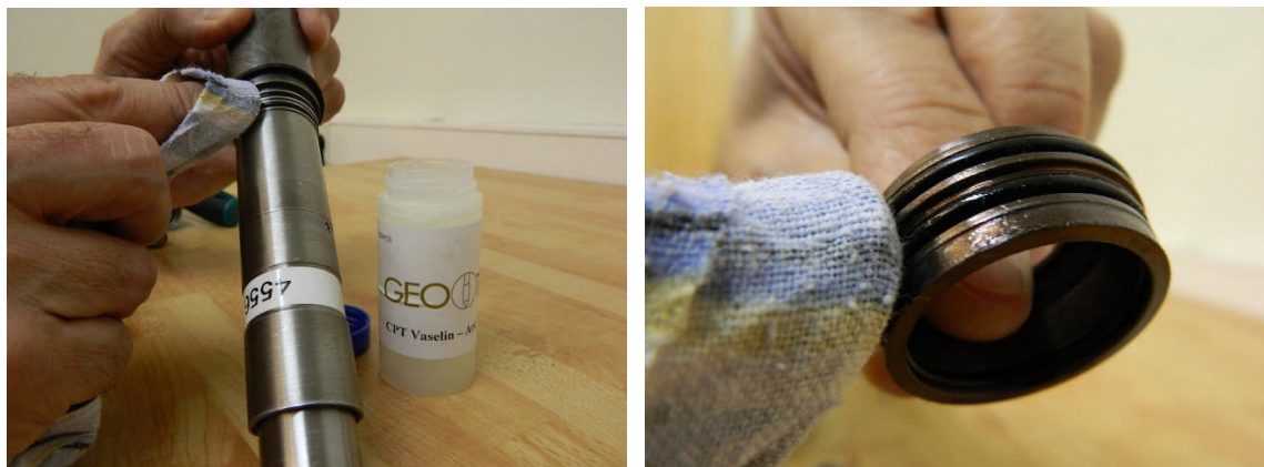
Fig. 32 – Mount the sealing rings and lubricate slightly with vaselin.
