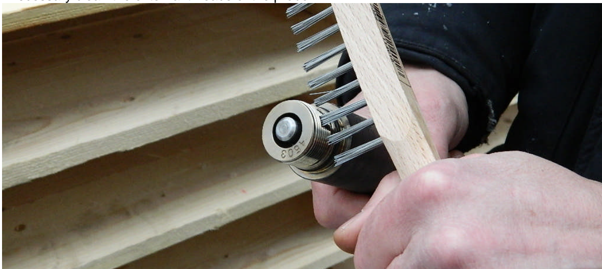
Fig. 30 – Cleaning the threads of the probe's end piece. Protect the contact area of the end piece from moist and water.
