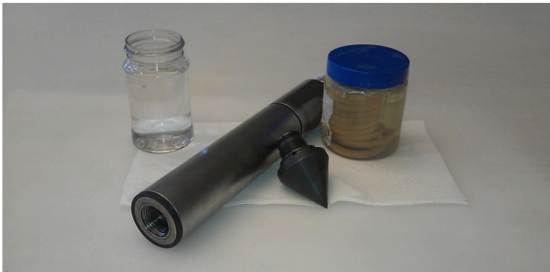
Fig. 18 – Use glycerine and saturated filter rings for de-airing the CPT GEOTECH NOVA probe
