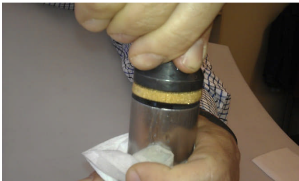
Fig. 19 – De-airing of CPT GEOTECH NOVA probe
